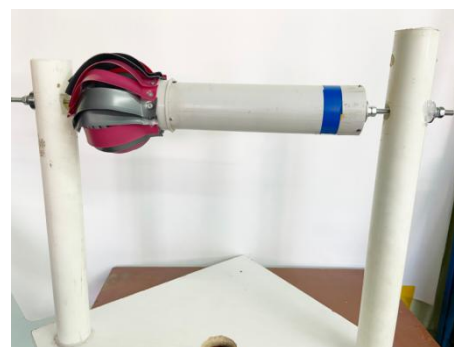
Figure 4. Experimental layout of a cylindrical blade with a plastic active deflector (made of polypropylene)
