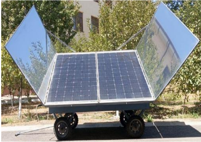
Fig. 5. Front view of a 1kW PV/TBD with a new type of cooling system.
