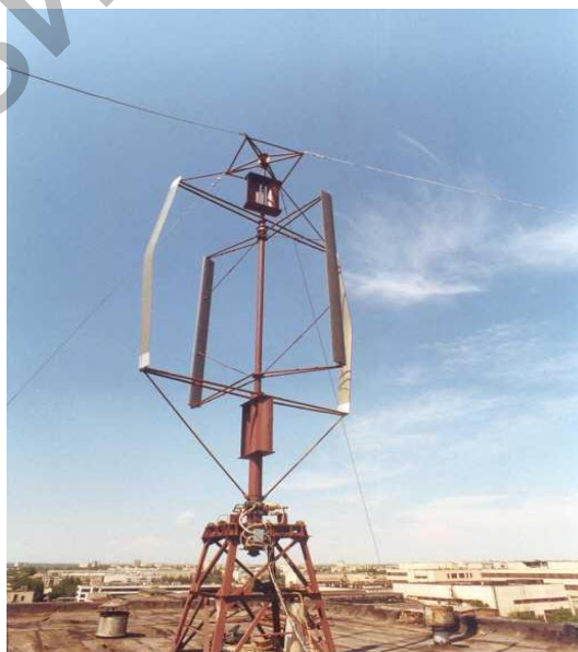
Fig.6. A semi-industrial specimen Bidarrieus-1 working in the mode with opposite rotation.
