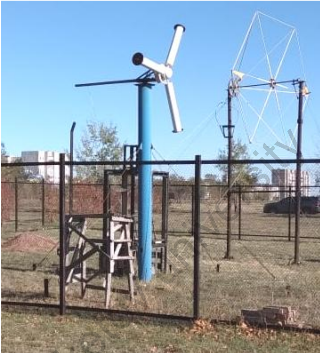
Fig.6.9. A prototype of a wind power plant with blades in the form of rotating cylinders a) front view, b) side view
