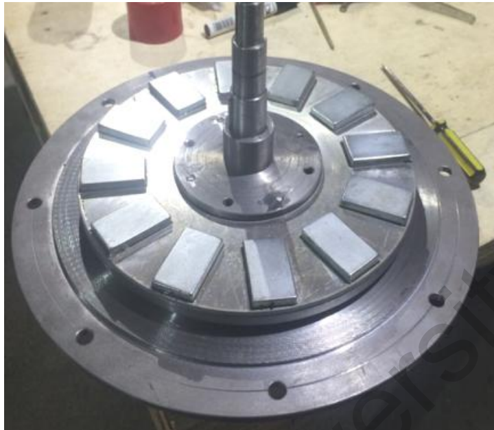
Fig.5.6.General view of a disk with 12 magnets
