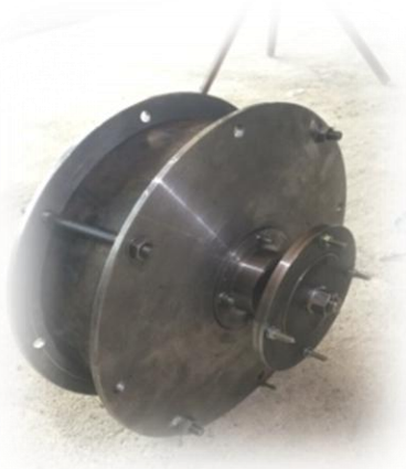
Fig.5.2. General view of the electric generator in the initial stage on permanent disk magnets
