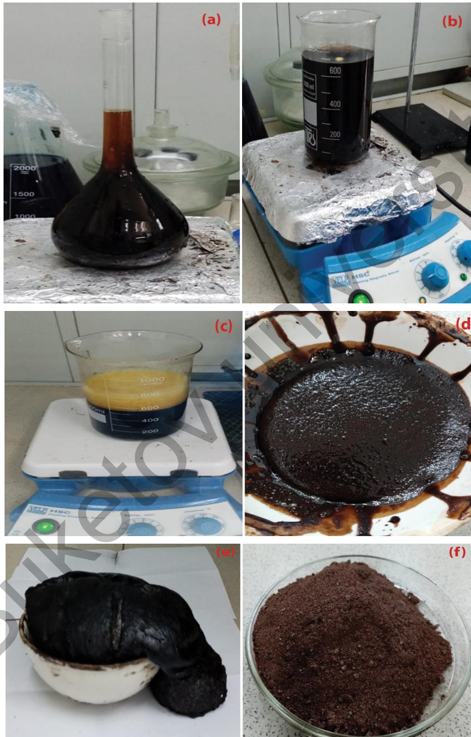
a — the metal salts aqueous solution in the flask; b — blending totally the whole mixture; c — heating the solution at 90^\circ\text{C} ; d — formation of a viscous liquid; e — formation of a fluffy carbonaceous pyrolyzed mass; f — obtaining nanoparticles ferrite
