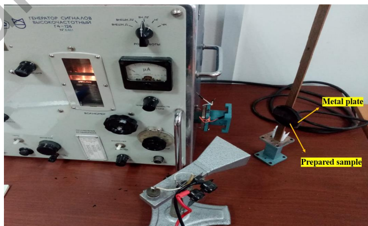
Figure 4. Experimental setup for measuring the reflected power of the EM waves by the free-space technique
