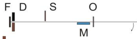
Fig.2. Scheme for measuring small-angle scattering: F is a focus, D is a primary diaphragm, S is a screen, M is a mirror, O is a sample.
