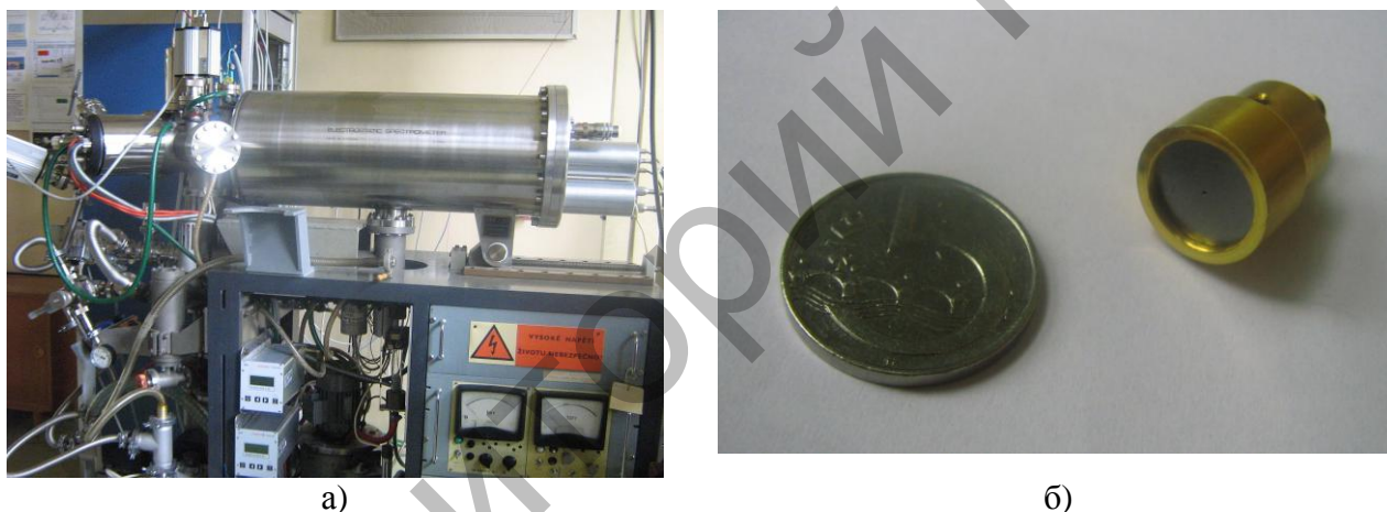
Fig. 2. The appearance of the ESA-12 electron spectrometer (a) and a radioactive disc-shaped source with the diameter of 8 mm (b).
