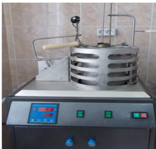
Fig.2. Installation for determining the ignition temperature
