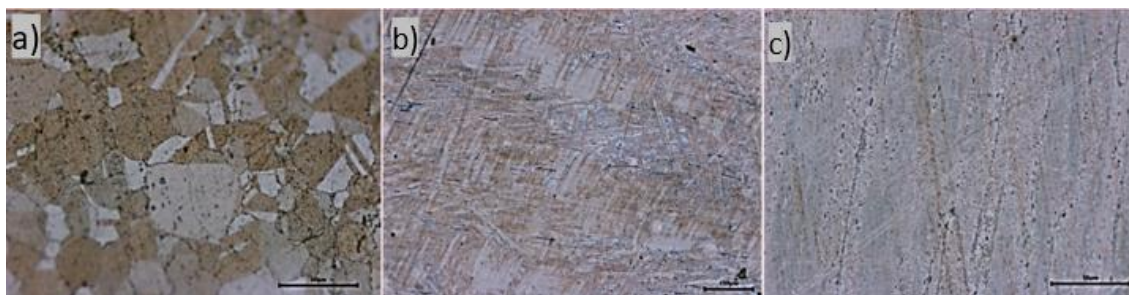
a — initial state; b — after quenching; c — after aging
