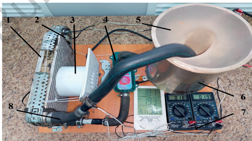
1- interior heater radiator; 2 - ultrasonic emitter; 3 - axial fan; 4 - circulation pump with heating element; 5 - filter; 6 - liquid reservoir; 7 - temperature control devices; 8 - rubber pipes
