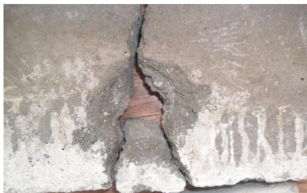
Fig.6. Break of the stone after drilling for 5 minutes ( h = 40\text{mm} )
