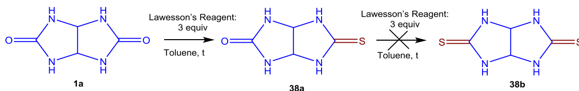
Scheme 28. The synthesis of monothioglycoluril 38a
