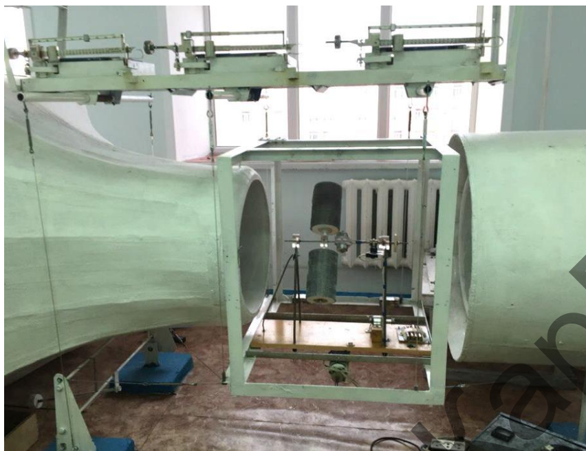
Fig.2. A model of a two-bladed wind turbine in the working section of a wind tunnel.
