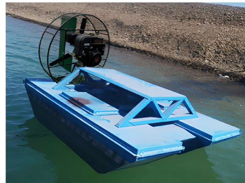
Fig. 2. Catamaran with an airboat installed
