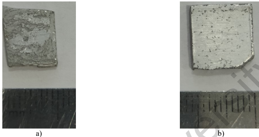
Fig.4. Photographs of the surface of samples exposed to alcohol solution of iodine for 72 hours: a) an untreated AMg2 sample; b) a sample treated with ozone for 6 hours.
