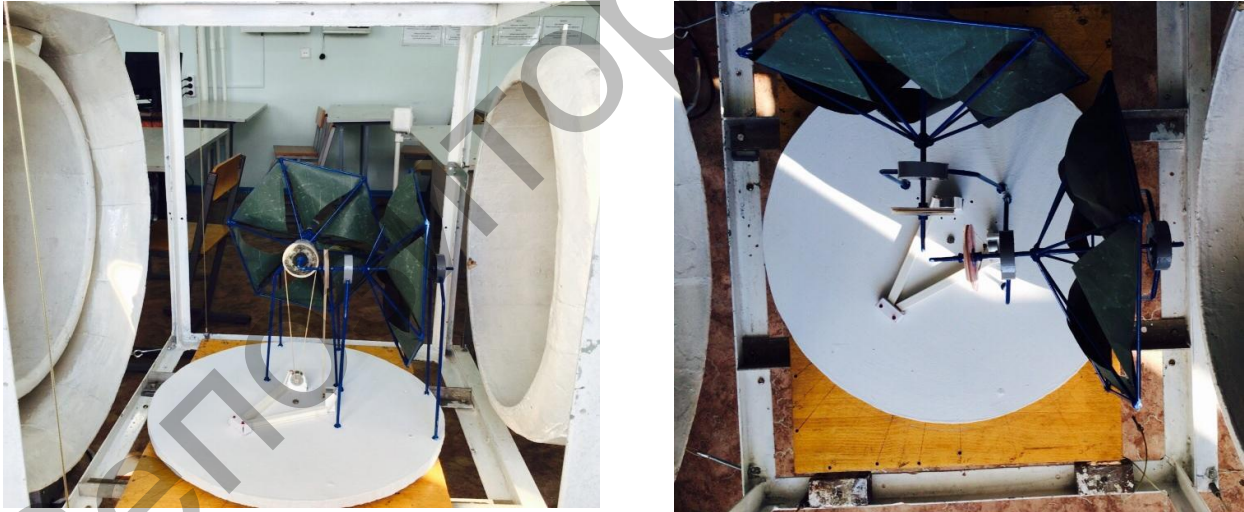
Fig.4. The overview of the reduced model of a double wind turbine in the operation area of a wind tunnel
