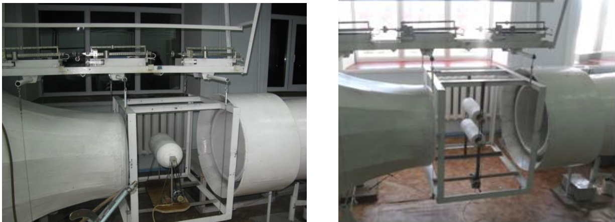
Fig. 4. The working part of the wind tunnel with a single (left) and with two (right) cylinders
