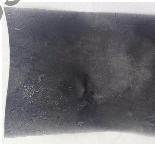
Fig.3. Appearance of a graphite film in a polymer matrix prepared by the second method.
