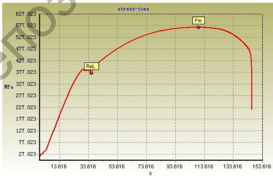
Fig.3. Diagram of the sample stretching 20GL steel, smelting No.226, grain score 9
