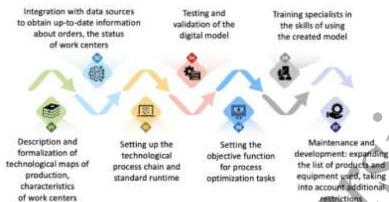
Figure 8. The stages of digital twin construction
