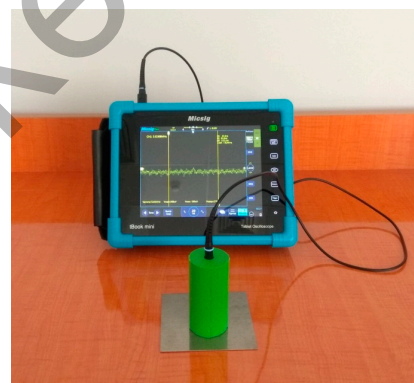
Figure 2. Device for measuring surface energy.
