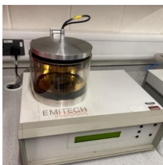
Figure 8. Appearance of the “Emitech K550X” installation
