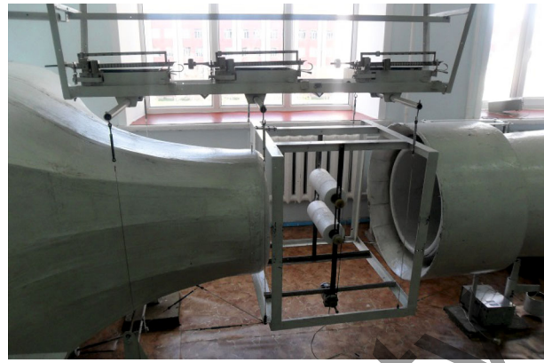
Fig. 2. General view of the working part of the wind tunnel with installed rotating cylinders being tested.
