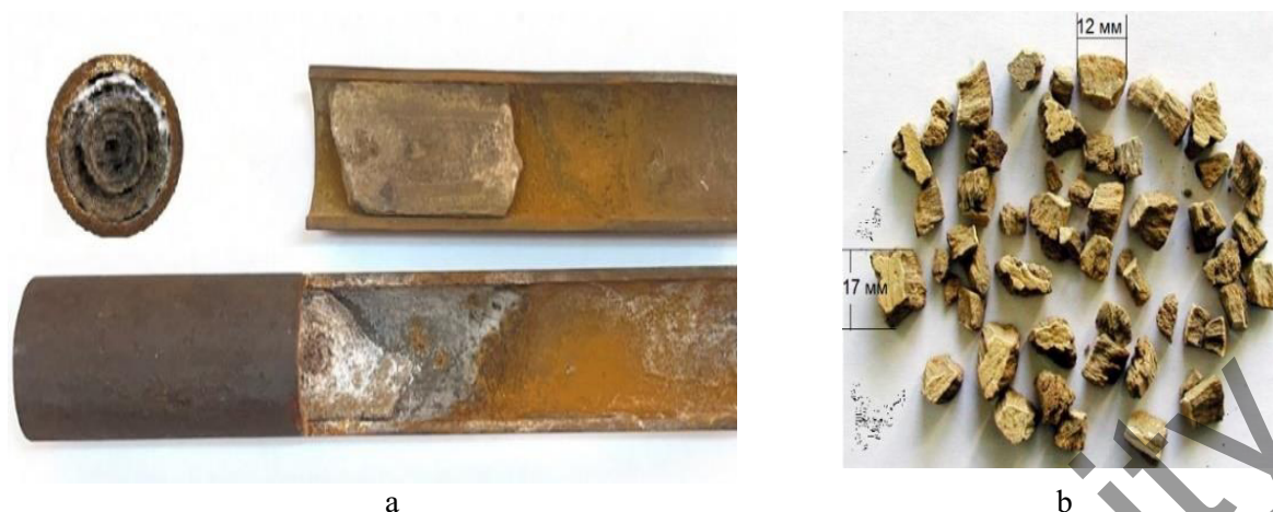
Figure 4. Samples of boiler pipes before and after cleaning using EHP — treatment: a) with hard deposits before processing; b) partially cleaned after processing, d = 51 mm
