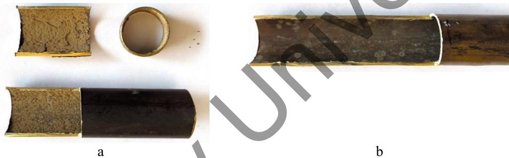
Figure 3. Samples of condenser pipes sections from CHPP-3, d = 24 \text{ mm} a) before processing; b) — completely cleared using the EHI effects.
