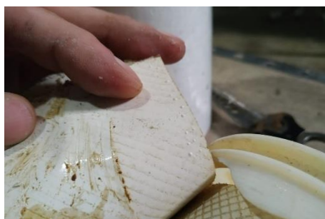
Figure 3. Photo of the membrane samples after the tests, without using EWTD
