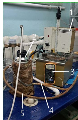
Fig. 1. Laboratory model for setting the temperature regime for melting fat from bone mass: 1 – thermostat; 2 – liquid heating tank; 3 – multimeter; 4 – water outlet tube; 5 – water supply tube
