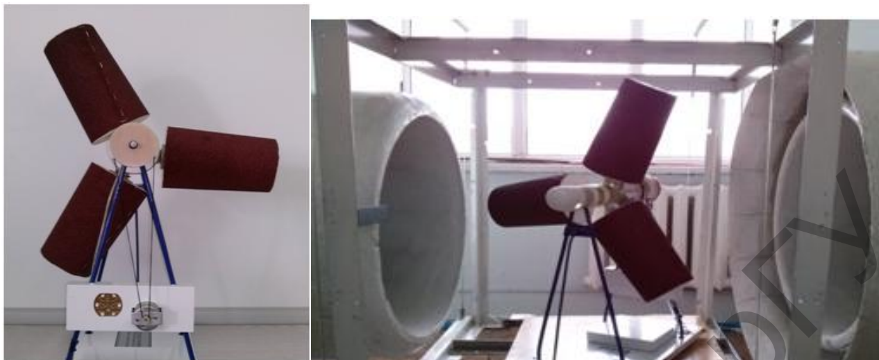
Fig.1. The model of the wind turbine with rotating cylinders of various cross-sections: a) a general view; b) in the working section of the wind tunnel.
