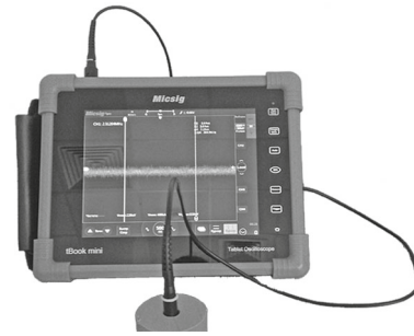
Fig. 1. System for measuring the contact potential difference of aircraft components.
