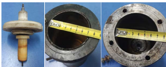
(b) positive electrode and metal chambers with an inner surface of a flat and hemispherical shape
