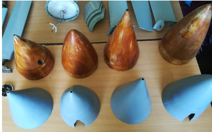
Fig.4. The components and corresponding fiberglass fairings.
