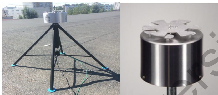
Figure 1. External view of the EFM-100 and its installation at ENU
