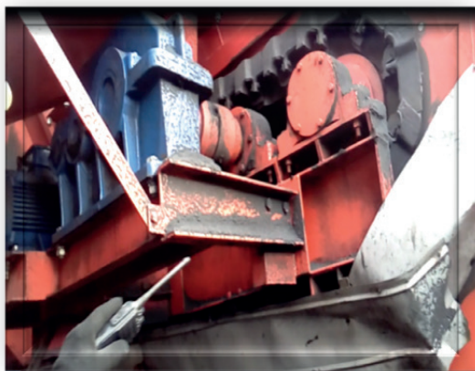
Figure 1 Electric plate drive feeder type KM PP 2-10-60
