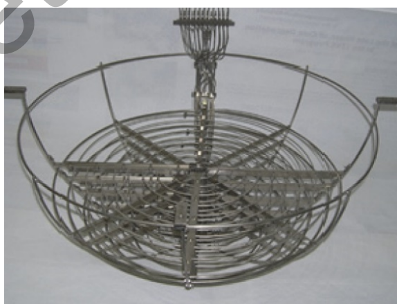
Fig. 6. Ohmic heater in LIVE experiment
