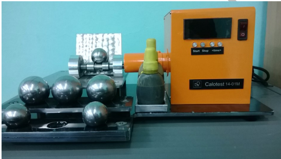
Fig.5. A device developed by us for testing materials and coatings for microabrasive wear
