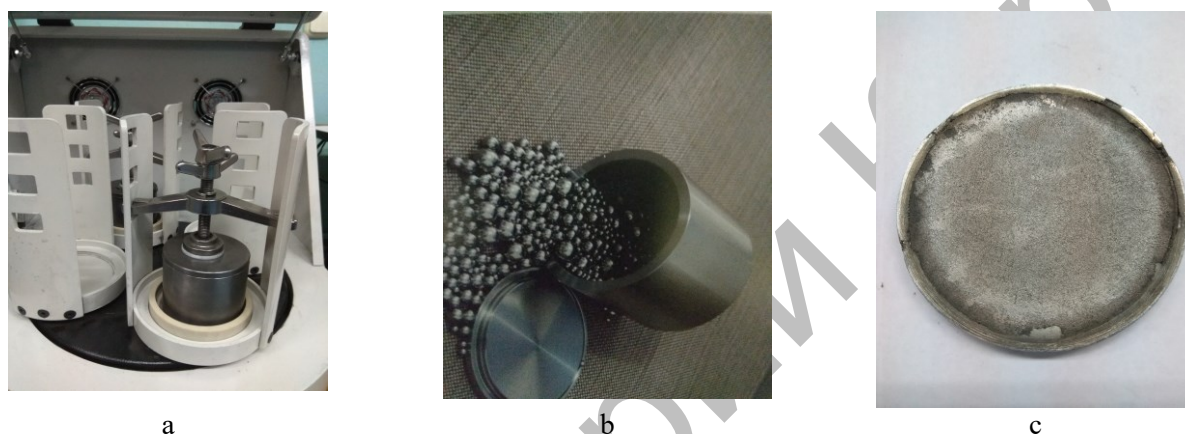
Fig.1. Magnetron target synthesis: a - planetary ball mill; b - micropowders of metals; c - finished target
