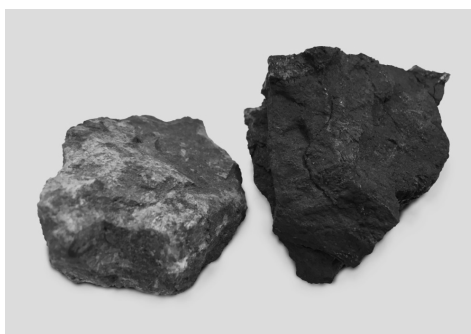
Figure 2. Samples of native (left) and calcined at 1000 °C
