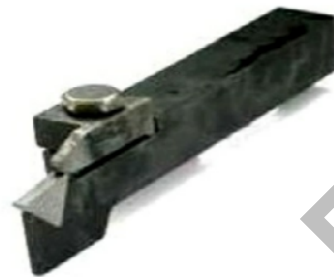
Figure 4. General view of cutoff tool with lateral mounting of MUP
