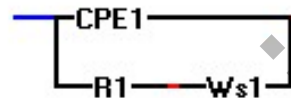
Fig.3. Equivalent electrical circuit, where R_1 is active resistance; CPE - constant phase element; W_{s1} is the “final” Warburg element characterizing the diffusion properties of the sample.
