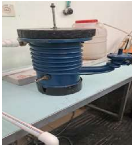
Figure 3. Working cell for separating fat from organic compounds
