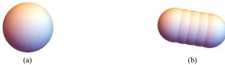
Figure 3. 3D model of generated aluminum alloy particles: a) sphere, b) elongated particle made of five overlapping spheres.
