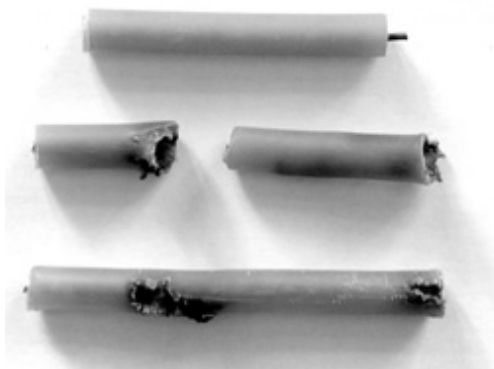
Figure 7. The electrode cable and its typical fractures in the course of operation
