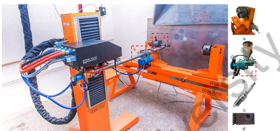
a — manipulator; b — powder dispenser; c — spark plug; d — dispensing plate
