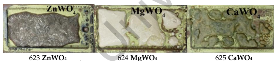
Figure 2. Photographs of \text{ZnWO}_4 , \text{MgWO}_4 , and \text{CaWO}_4 ceramic samples synthesized under the influence of an electron flux with E = 1.4 MeV, P = 15 kW/cm 2 .
