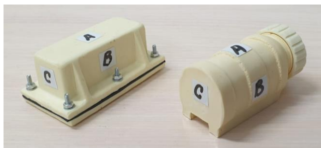
Fig.2. Compression load sides: left – rectangular housing; right –cylindrical housing
