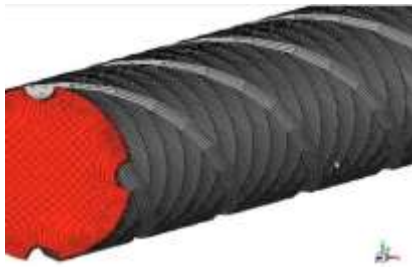
Figure 1. Calculation grid of the pipe with windings
