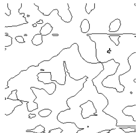
Fig.7. Fractal structure of the Mn-Fe-Cu-Al coating
