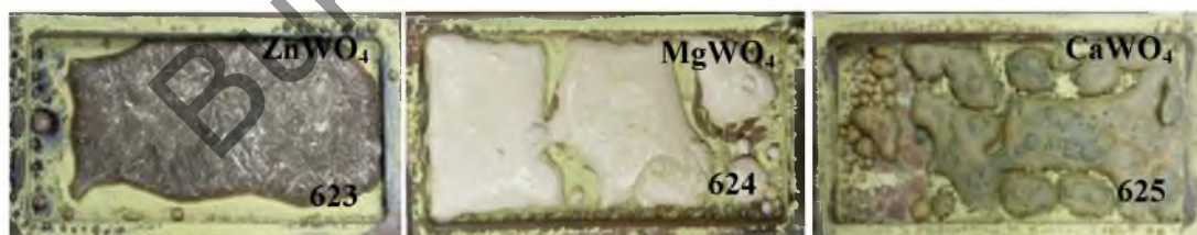
Figure 4. Photos of samples of synthesized ceramics ZnWO 4 , MgWO 4 , CaWO 4
