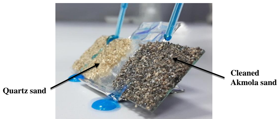
Figure 10. The microfluidity of water with blue dye on surfaces of superhydrophobic sands of quartz and Akmola region
