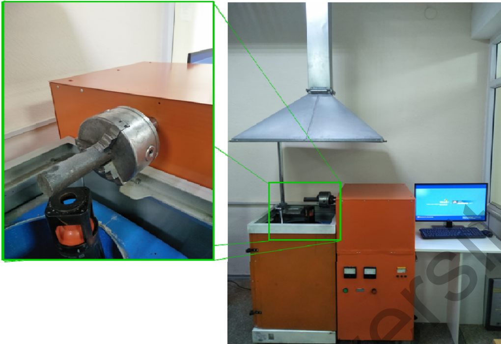
Figure 4. The general view of the installation thermal cyclic electrolytic plasma hardening
