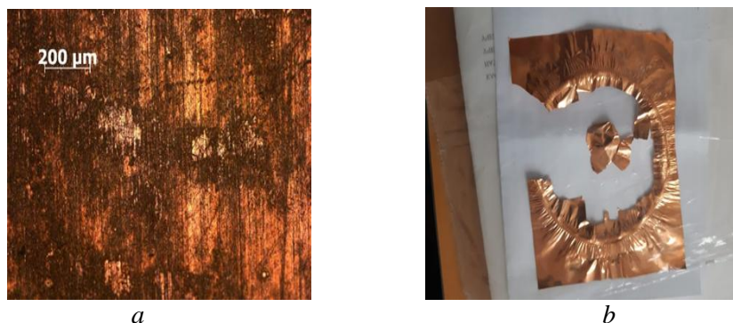
Figure 3. Fragments of a sample of copper foil before (a) and after (b) the magnetic field destruction test. The micrograph (a) shows traces of rolling, which confirms the X-ray diffraction picture
