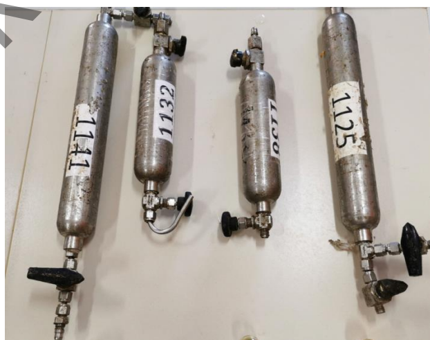
Figure 4. Pressurized cylinders for a polymer solution sampling at the wellhead
